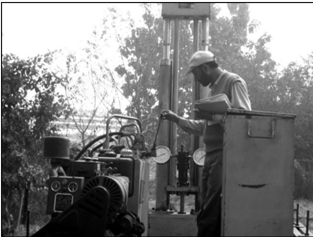
Figure 4 : Static Cone Penetration Tests
